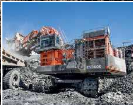
EX ultra-large excavators
