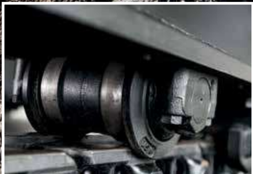
Redesigned lower roller prevents mud entering and causing damage.
